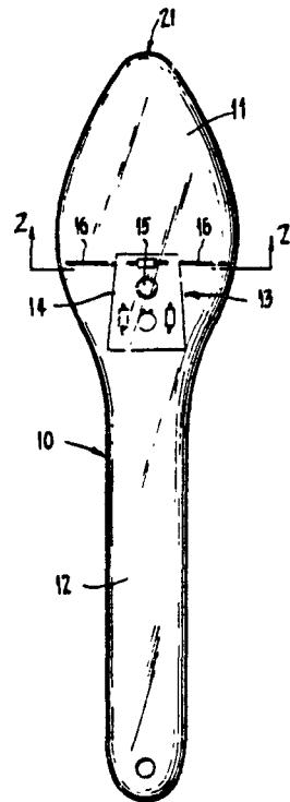
ing the dipoles integrally in a solid block their resonant frequency is altered and thus the length of the dipoles and consequently the size of the detector is reduced. A method of constructing a detector is also claimed.
